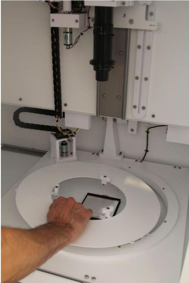
Place the desired sieve support frame, then take the 3 fasteners.
