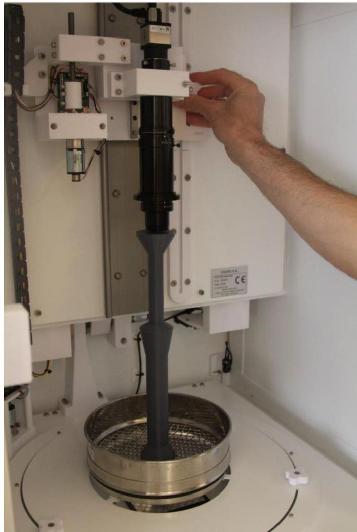
For calibration, be sure to remove the lens when place the small shim.
